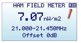
• The 30dB Attenuator **A30** icon and **LNA** low noise preamplifier icon are now included in main screen (Spectrum Analyzer and HAM Field Meter modes) to visually indicate when these options are enabled. No icon is displayed for the DIRECT default mode. For Expansion boards with support for 60dB Attenuator icon **A60** is also available.
